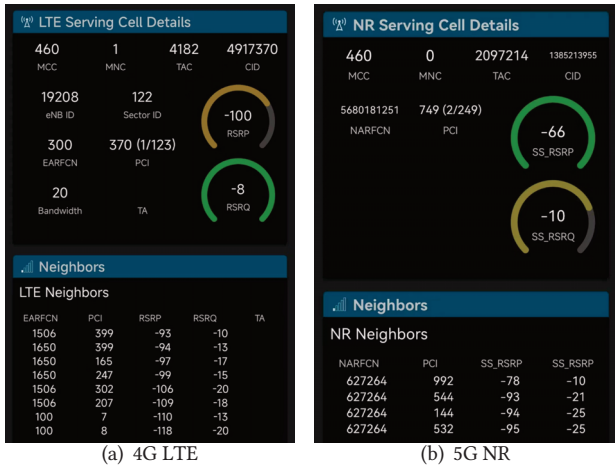
Figure 1: User Measurement Data (UMD) in 4G LTE and 5G NR network, recorded by a commodity app “Network Survey [2]”.
