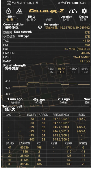
Fig. 9. An application to record the information of cellular stations. EARFCN denotes the local indicator of each neighbor station.
