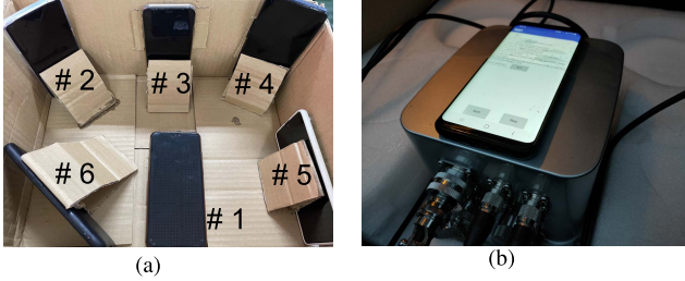
Fig. 4. Dedicated measurement by a mold with six smartphones. (a) Mold with six phones. (b) Dedicated IMU device.
