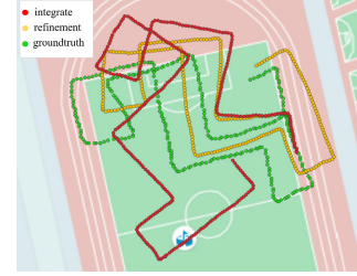
Fig. 11. Drift correction example. By using drift correction, the trajectory is closer to the groundtruth than the raw trajectory.
